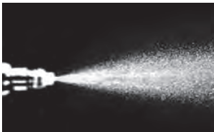
Injector spray pattern after P.i. treatment.
