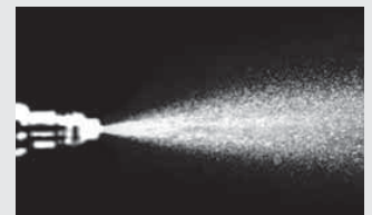
Injector spray pattern after P.i. treatment.
